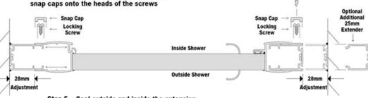
Step 5 - Seal outside and inside the extension profiles, along the bottom of the sill rail and where the head and sill rails meet the jambs, using a clear antimould silicone sealer
